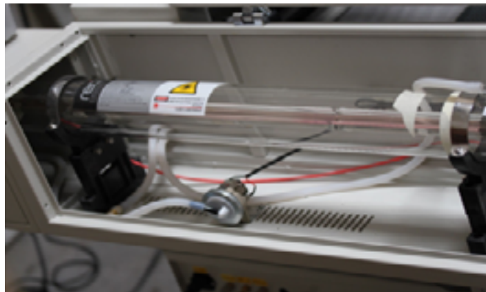
Laser tube properly installed
