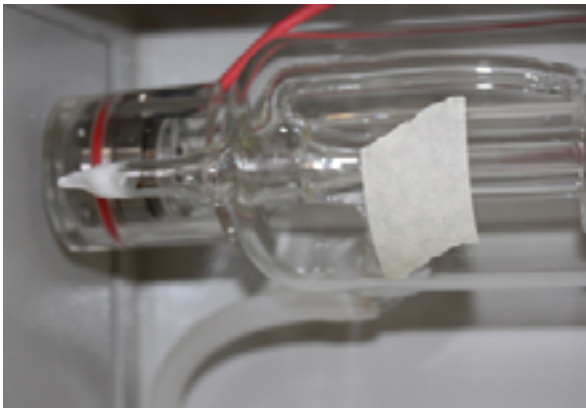
Left end of laser tube with red wire and plastic cap installed correctly.
