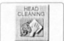
Press the SET button and execute cleaning by selecting HEAD CLEANING from OTHERS on the initial screen.
