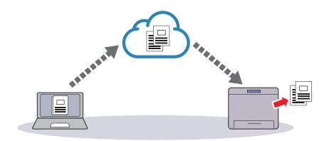
Google Cloud Print version 2.0 sends the print data to the printer either via Internet or via local network. This version is recommended for the environment where the Internet connection cannot be used.
