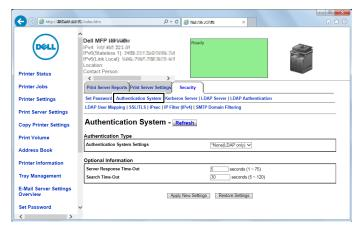
2 From the Authentication System Settings drop-down menu under Authentication Type, select LDAP as the authentication method, and then click Apply New Settings.
