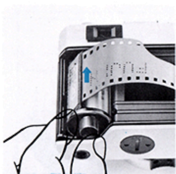
2. Hold the cartridge with the spool head pointing to the bottom of the camera and fit the Film Rewind Crank Shaft into the hole in the opposite end of the cartridge. The cartridge will now fit snugly in the Film Chamber.
