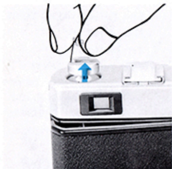
1. Lift the Film Rewind Crank.
