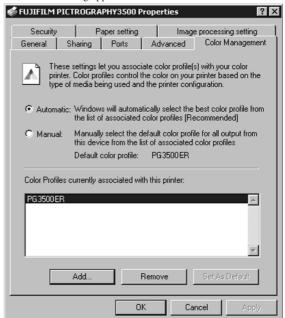
Here, you can add or delete profiles related to the printer. Note that profiles for the PICTROGRAPHY 3500 were added when the printer driver was installed. Under normal conditions, these settings should not be altered.
