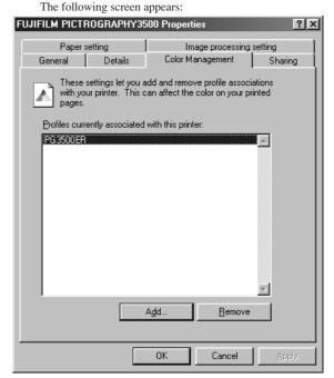
Here, a profile related to the printer may be added or deleted. The profiles for the PICTROGRAPHY 3500 are added during printer driver installation. Do not modify the settings unless absolutely necessary.
