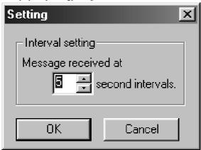
In the [Interval setting] field, specify the interval at which to check printer (server) status.
