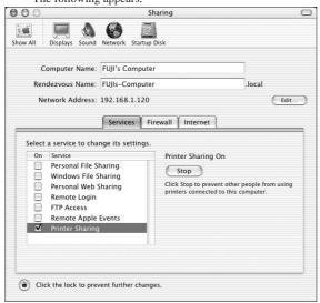
Mark the [Printer Sharing] check box with a " √ " and close the [Sharing] window.
