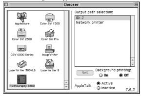
Click [ID: n] (the SCSI-ID value of the connected PICTROGRAPHY 3500 is displayed in the area of n) of [Output path selection:].
