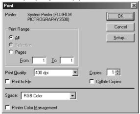
After verifying that [PICTROGRAPHY3500] appears in [Printer:], set up the necessary items and click the [OK] button. Printing is executed.
