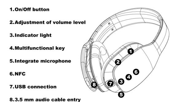
Before using the headphone, you must fully charge the battery and connect the headset to your respective Bluetooth device.
