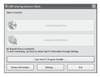
2. Click "Settings" button, then click "Searching for Host PC on the network" to auto search Host PC on the network and type in "Shared Drive name on the destination" which appears on setting screen of "ODD sharing feature Client". After select the desired Application Behavior, Click "OK" to confirm.
