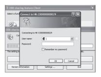
For user's PC cannot access Internet Network/location or at places without wireless network connected, user can establish ODD sharing network by set up a wireless ad hoc network, please ensure you have switched on the wireless LAN function of both Client and Host PC.
