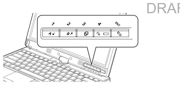
Figure 32. LIFEBOOK T901 Tablet PC Security/Tablet PC Buttons
