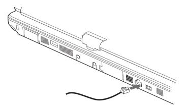
Figure 41. Connecting the LAN
