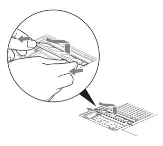
Figure 40. Removing a Memory Module
