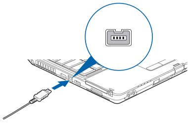
Figure 43. Connecting an IEEE1394 Device
