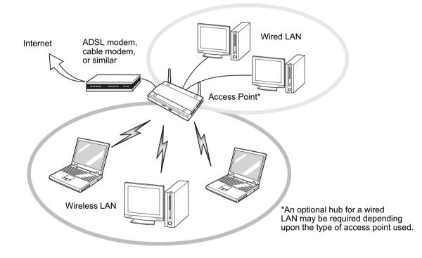
Figure 52. Access Point (Infrastructure) Mode Network
