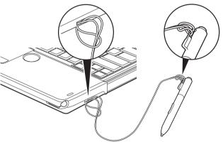
Figure 29. Installing a Pen Tether
