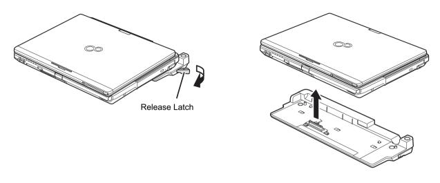
Figure 47. Unlatching the Port Replicator
