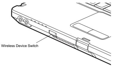
Figure 53. Wireless Device On/Off Switch Location
