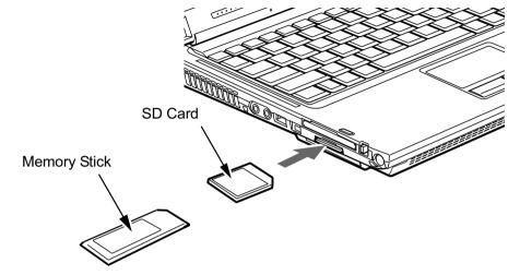
Figure 35. Installing a Memory Stick or SD Card
