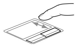
Figure 22. Scrolling with the Scroll Strip
