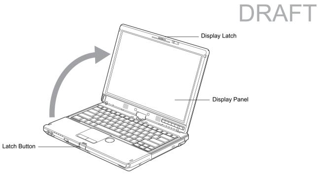
Figure 8. Opening the Display Panel
