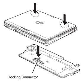
Figure 46. Attaching the Port Replicator
