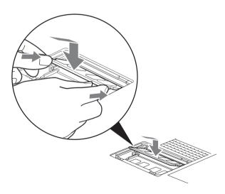
Figure 39. Installing a Memory Module
