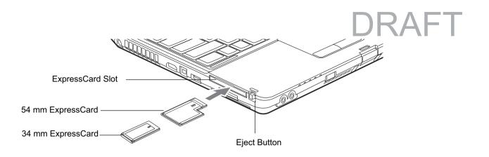
Figure 36. Installing/Removing ExpressCard
