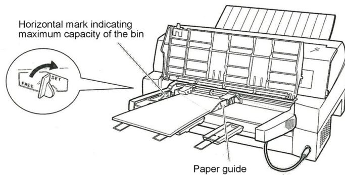
**Loading the cut sheet feeder (Front feed)**
