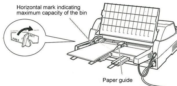
**Loading the cut sheet feeder (Rear feed)**
