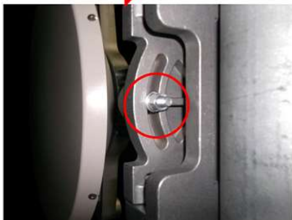
Elevation Fixing Bolt (Antenna front side)
