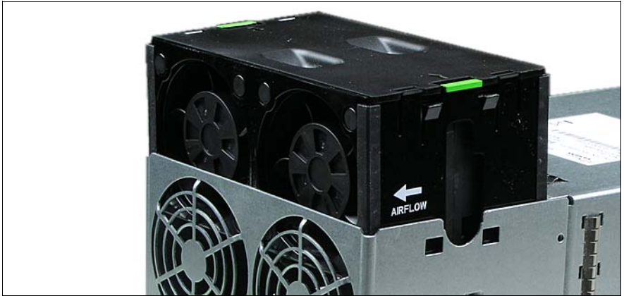
Figure 57: Installing a fan unit
