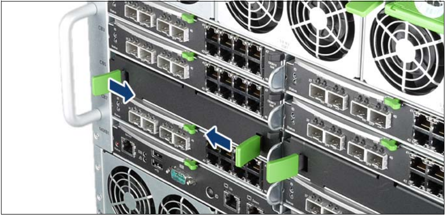
Figure 43: Removing a dummy connection blade module
