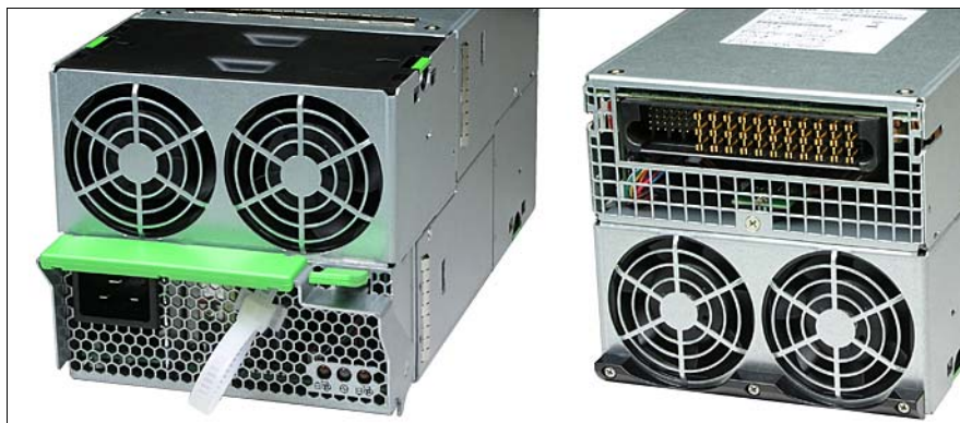
Figure 55: Fan units in a power supply unit
