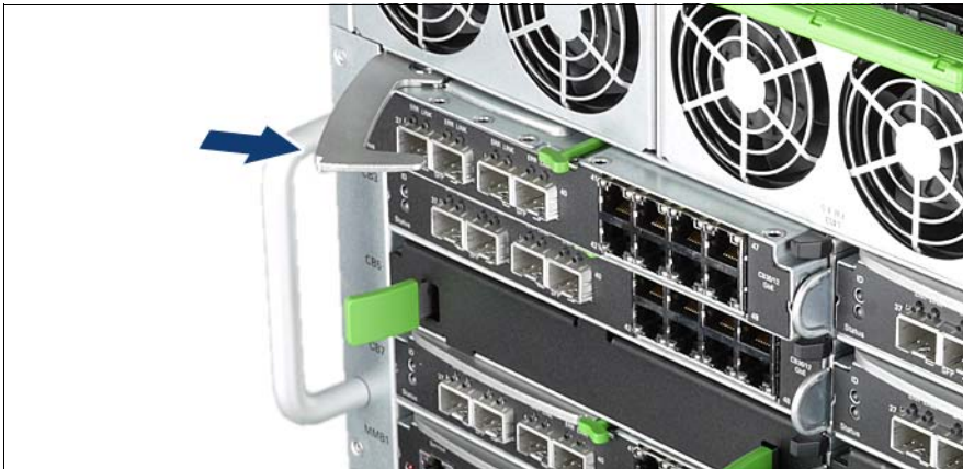
Figure 45: Locking the connection blade
