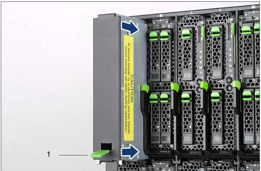
Figure 25: Installing a dummy server blade module
