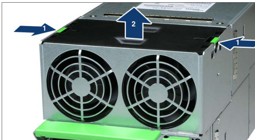
Figure 56: Removing a fan unit
