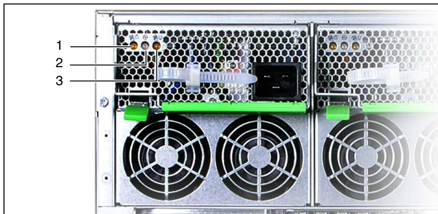
Figure 16: Indicators on the hot-plug power supply unit
