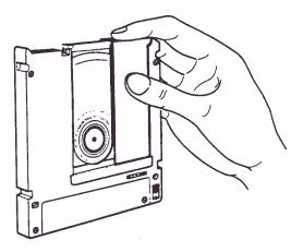
Figure 5.6 Cleaning procedure (1)
