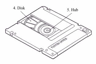
Figure 5.4 Optial disk cartridge
