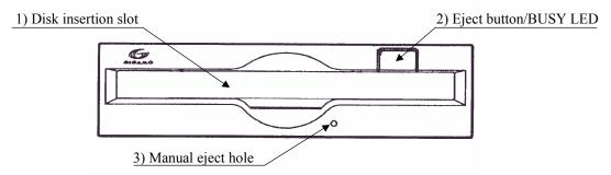
Figure 5.1 Optical disk drive front view (with panel)
