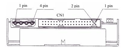
Figure 3.9 Connector and terminal locations
