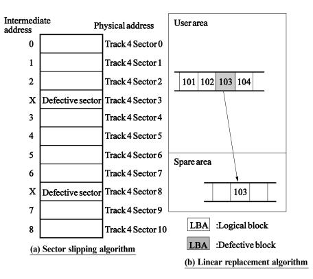
Figure 2.2 Algorithms for alternate processing
