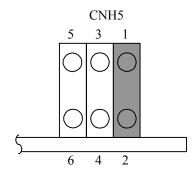
Figure 3.14 Cable select mode setting
