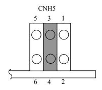
Figure 3.13 Slave device setting
