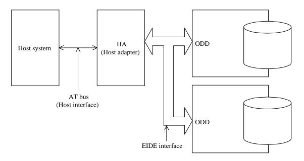
Figure 1.6 System configuration with two optical disk drives
