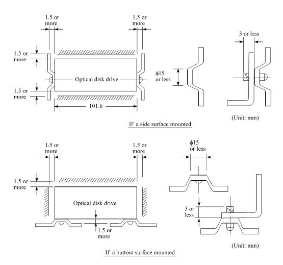
Figure 3.6 Mounting frame structure
