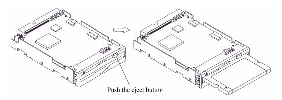
Figure 5.3 Removing cartridge
