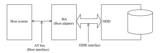
Figure 1.5 System configuration with one optical disk drive
