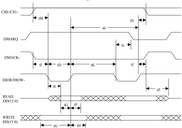
4.7.2 Multiword DMA data transfer timing
