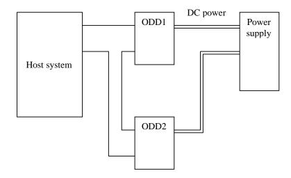
Figure 3.10 Cable connection diagram
