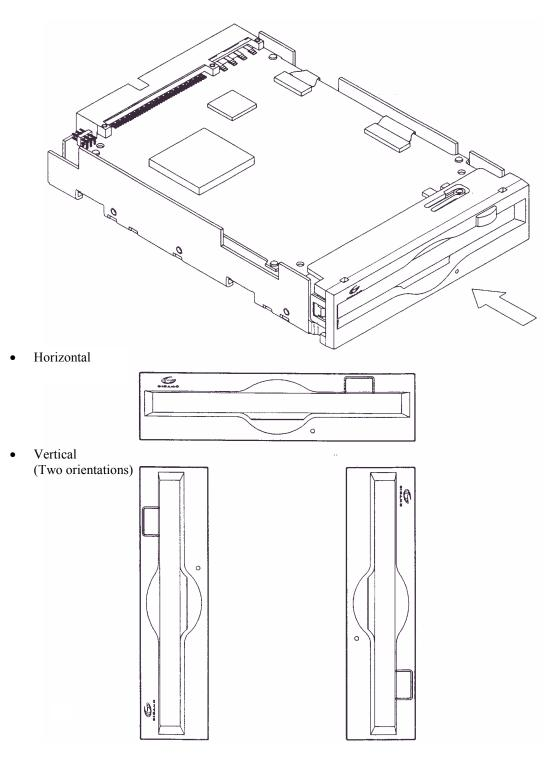
Figure 3.4 Installation directions
