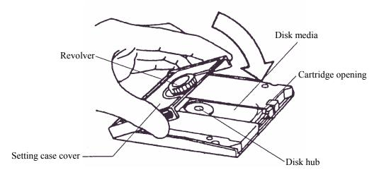
Figure 5.8 Cleaning procedure (3)
