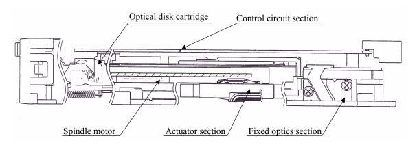
Figure 1.3 Optical disk drive configuration
