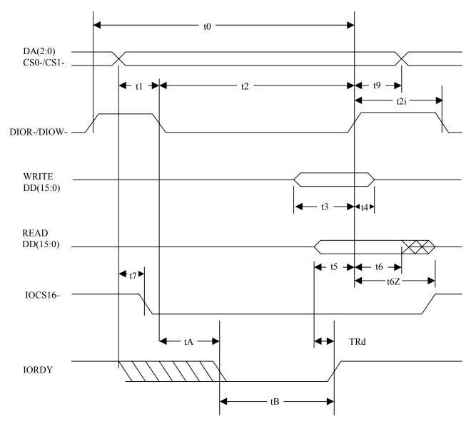
Figure 4.2 Register/PIO data transfer
