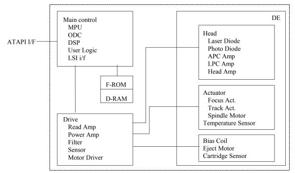
Figure 1.4 Control circuit section block diagram
