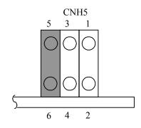
Figure 3.12 Master device setting
