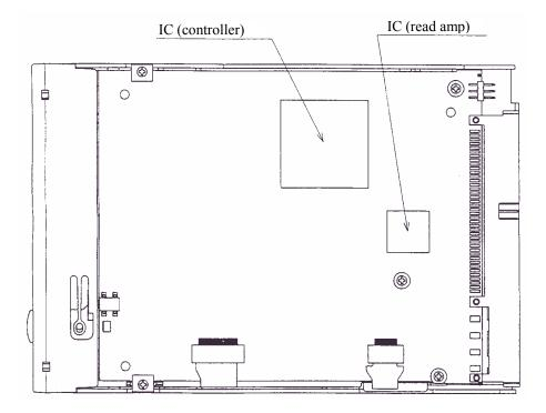
Figure 3.1 Surface temperature measurement points
