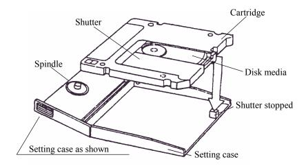
Figure 5.7 Cleaning procedure (2)
