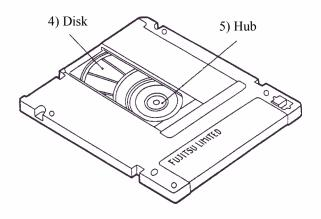
Figure 2.1 Optical disk cartridge
