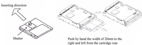
right and left from the cartridge rear center, to the position shown at right.
