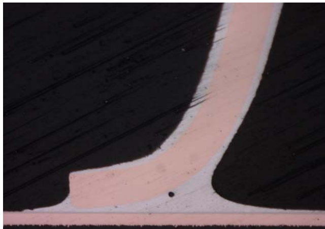
B) Paste : Sn-Ag-Cu Lead Frame : 42-Alloy Reflow Temperature :240°C
