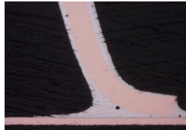
B) Paste : Sn-Ag-Cu Lead Frame : 42-Alloy Reflow Temperature :240°C
