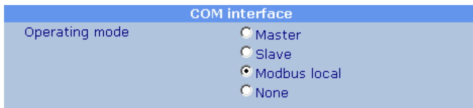
Interface settings for Modbus access
