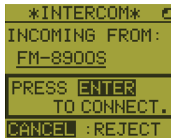
Off hook condition
