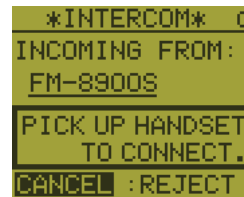
On hook condition
