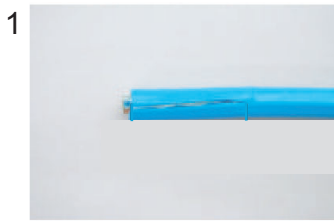
Expose inner vinyl sheath.
