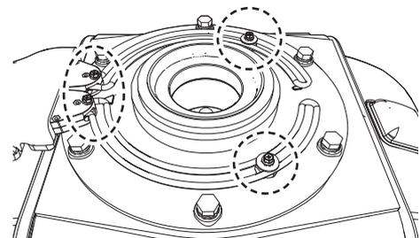
in the following figure. Pass the de-icer power cable through the locking wire saddles (1) to (6) and it to the front side.
