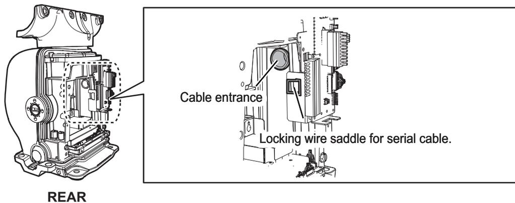
6. Attach the appropriate WAGO connectors (pre-attached) to the serial cable, and then connect the serial cable to the RF-TB Board as shown in the following figure. For how to connect the WAGO connector, see "WAGO connector" on page 2-6. For pin arrangement, see the interconnection diagram at the back of this manual.
