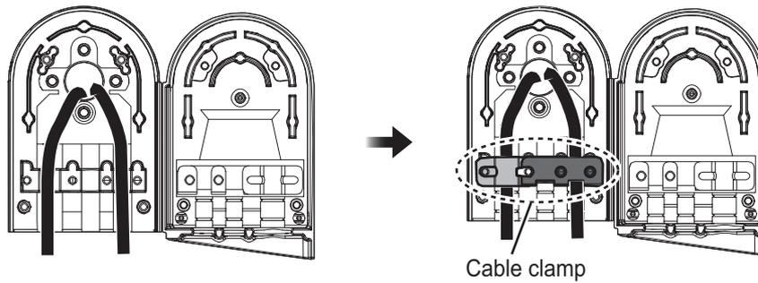
9. Coat the hinge with the supplied adhesive for hinge waterproof then close the cable entrance cover. Fix the cable cover with four screws, then coat the screws with the supplied adhesive.
