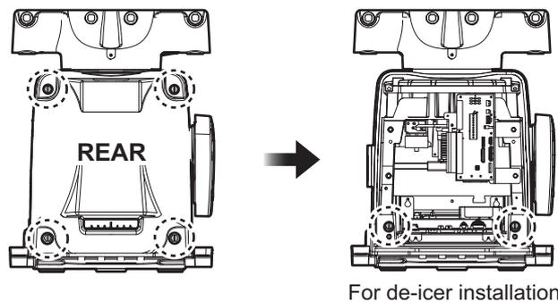
**Note 1:** The cable for the performance monitor is connected between the rear cover and the RF-TB Board in the antenna unit. Open the cover slowly to prevent damage to the cable and connector.
