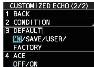
When [ACE] is activated, the [SEA] box and [RAIN] box are gray colored and cannot be adjusted, and the echo averaging function is disabled. The [GAIN] box changes to [GAIN ACE], as shown in the figure below.
