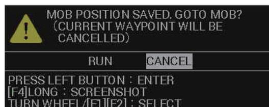
To navigate directly to the MOB, select [RUN]. A course line appears between your vessel and the MOB symbol, on the screen. The line represents the shortest course to the MOB and the arrows on the line indicate the direction of travel.
