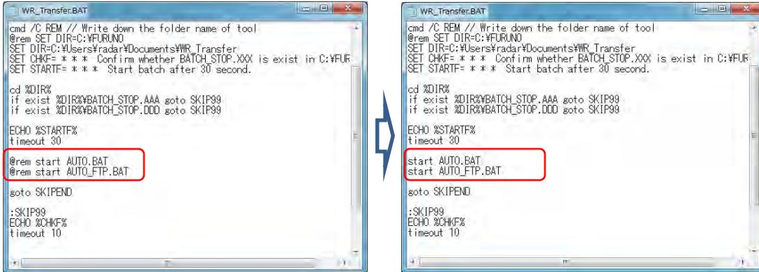
Figure 4.10: Sample of WR\_transfer.bat (Before -> After)
