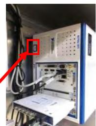
2. Shut down the circuit breaker in the storage box.
