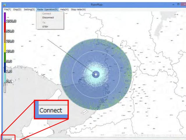
RainMap will display [Connect] at the bottom-left of screen when the Antenna Unit (ATU) and Display Processing Unit (DPU) are connected and communicating.
