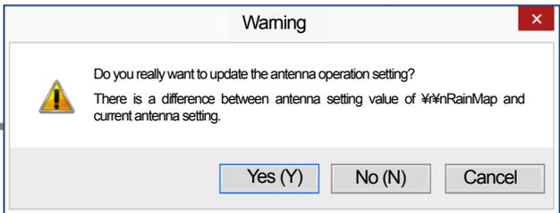
If [Yes] clicked, antenna will initialize and will indicate the message below. Radar will start TX operation after initialization completed.
