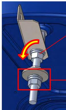
Turn the lifting tool outward by slightly loosening M16 hex nut.
