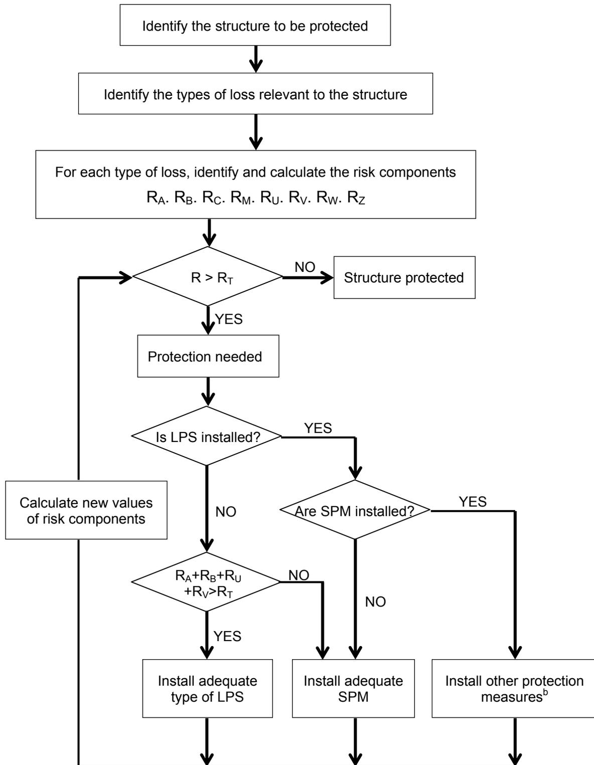
Figure A-1: Procedure for deciding the protection requirements and selecting protection measures
