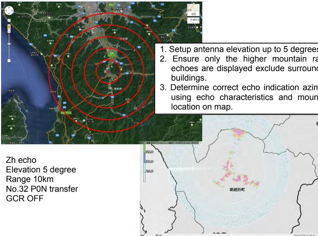
**Note:** Elevation angle written here is one example. It depends on geographical feature where radar is located. For another example, if it is in a flat country like Denmark, a water tower in Lund, and Sweden, it used -1 degree, 10 km range and was able to detect coastline and the city borders of Copenhagen.
