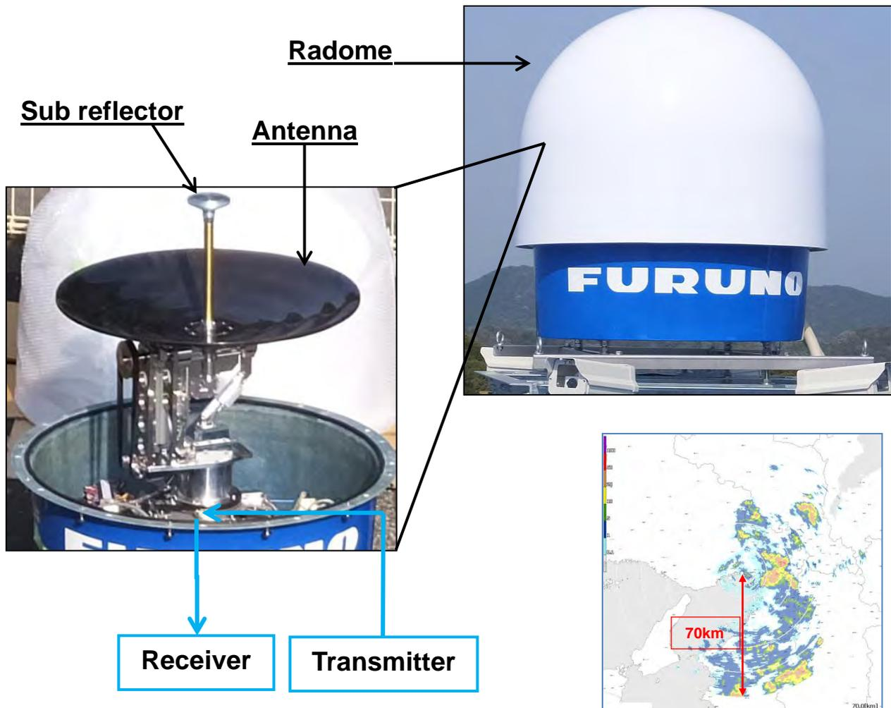
**Antenna:** The main purpose of the antenna is to focus the transmitted power into a small pencil beam and also to receive and collect the returned signal.
