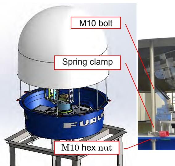
10. For reducing from the wind-induced movement, fasten the spring clamp above the base flange and tighten bottom hex nut by hand.
