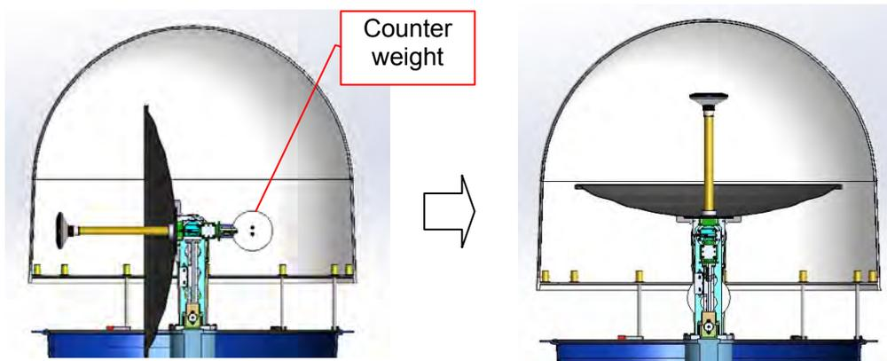
8. Lift up the top of radome until the M10 hex nut contacts radome base flange.
