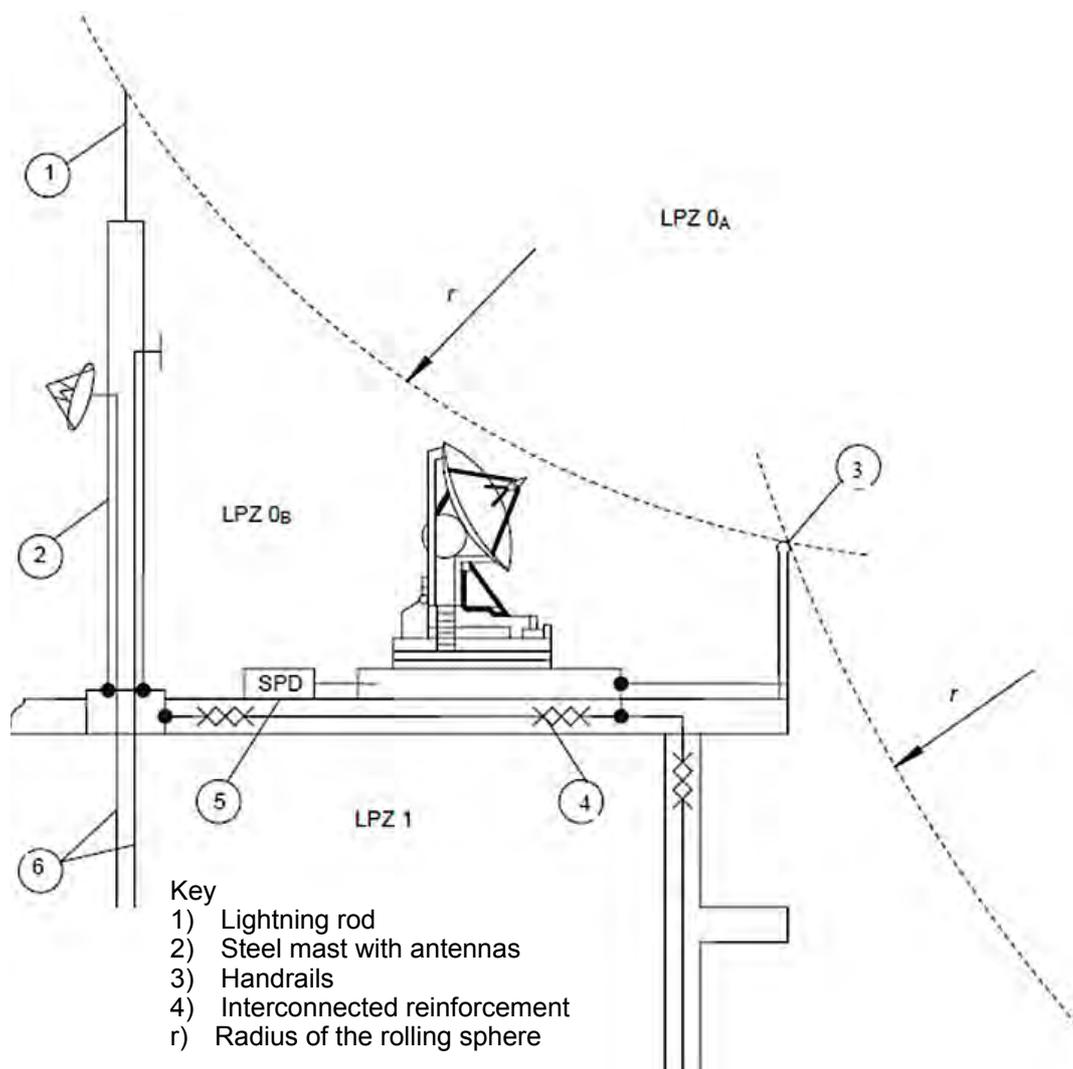
Figure A-3: Protection of a building and other external equipment (IEC 62305-4)
