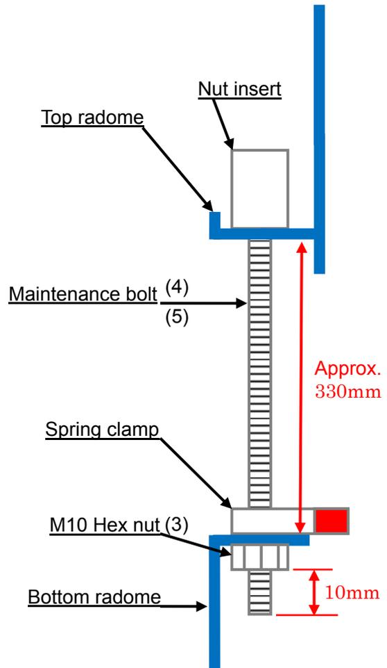
Ensure the radome remains level when adjusting maintenance bolt lengths.
