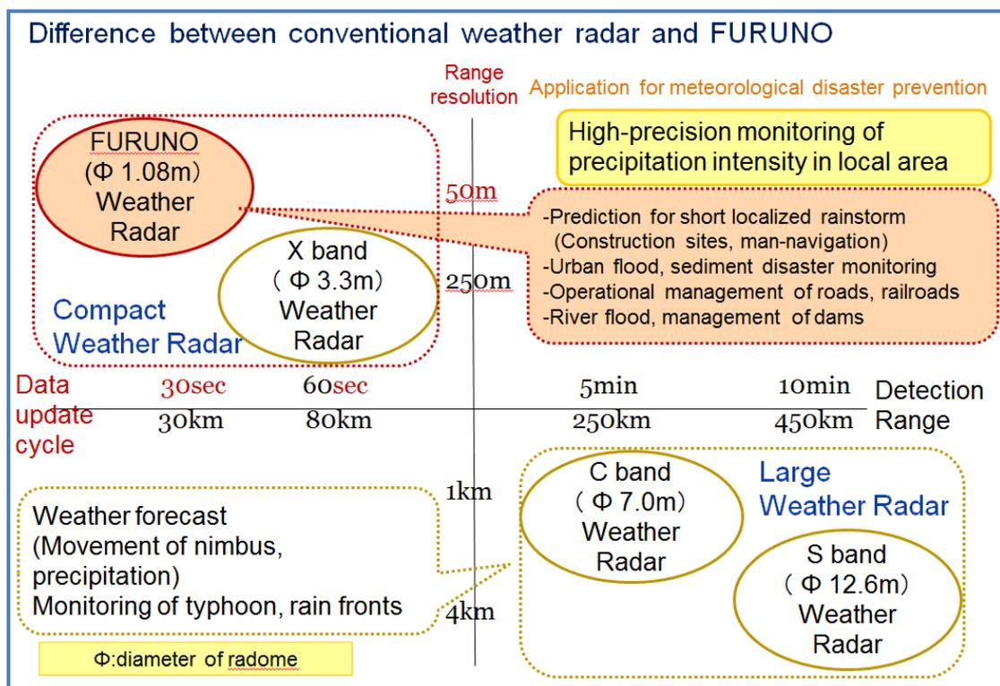
Figure 1.1: 3 general types of weather radar band
