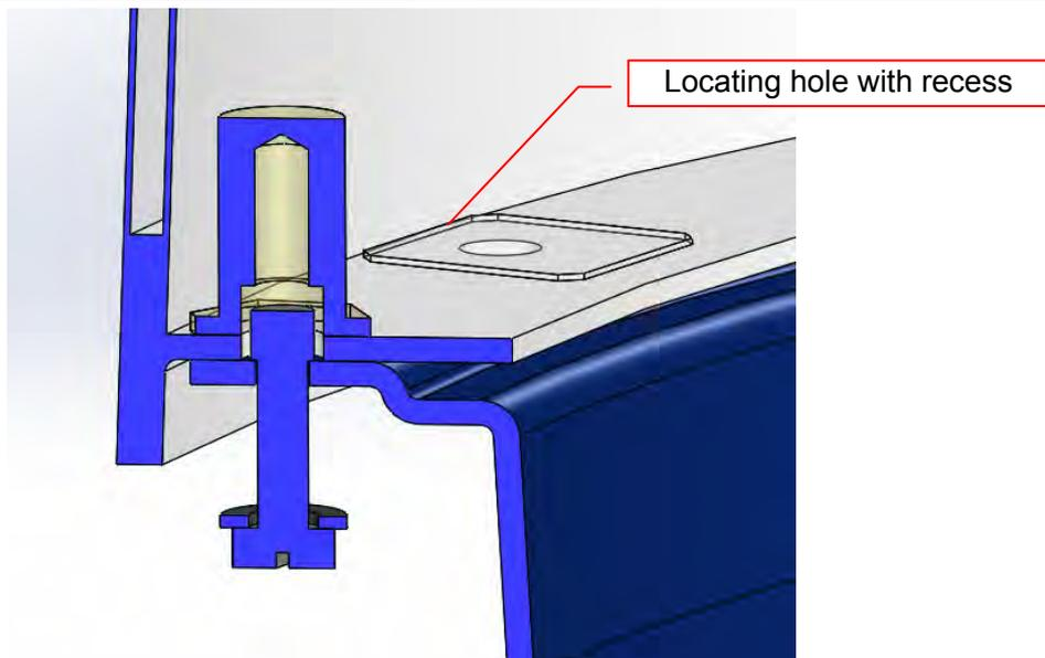
Figure 5.3: Before rotating top of radome
