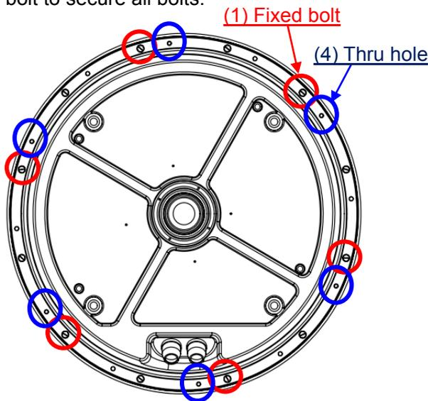
Image 5.1: Bottom view of radome (6 maintenance bolts)
