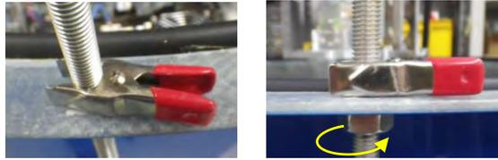
Figure 5.6: Fasten properly by spring
