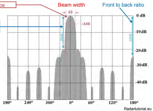
Figure 1.6: The same antenna pattern in a rectangular-coordinate graph
