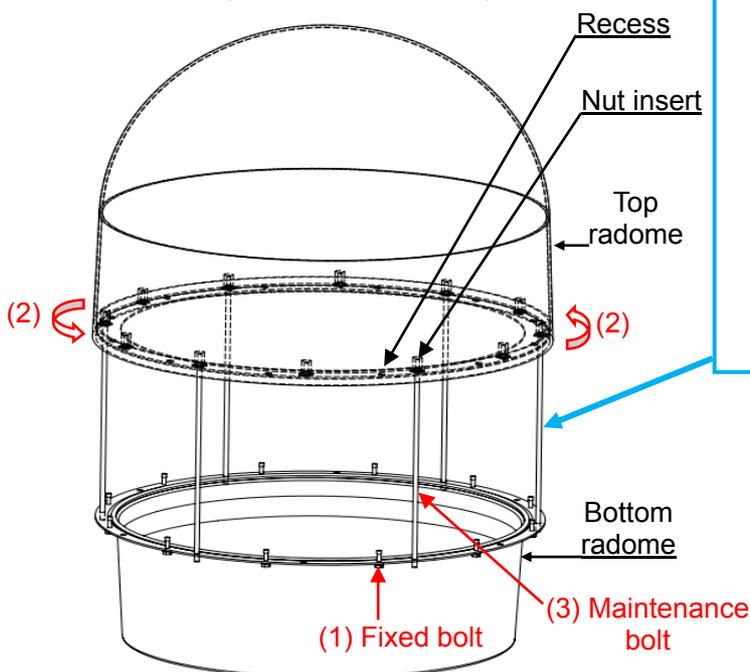
Image 5.2: Side view of radome (6 maintenance bolts)
