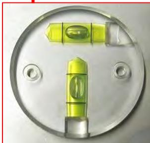
Adjust level with using the bubble level installed under the radome. The bubble must be in the center between lines. If the bubble is on the line or over the line, it means the angle is over 0.3 degrees. The level adjustment will be completed after all M16 hex nuts are tightened.
