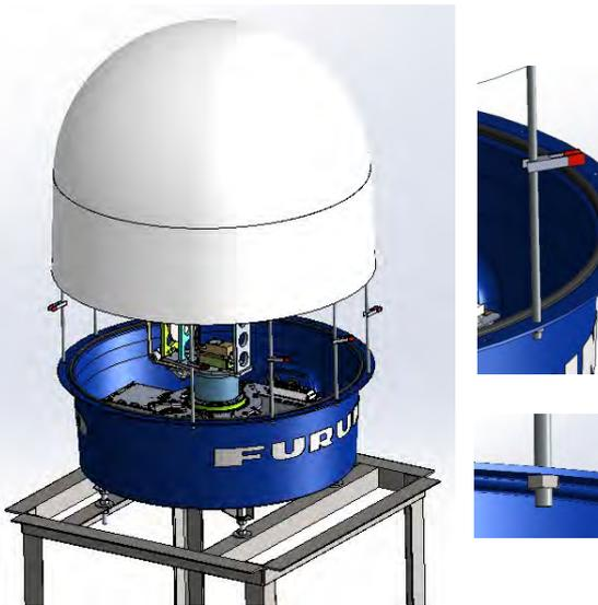
9. Fasten the spring clamp above the base flange.
