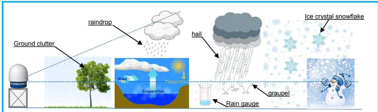
The area sampled by the radar increases with distance. The wider the beam the greater the likelihood of sampling a mixture of precipitation types and also a greater the likelihood of sampled both inside and outside a cloud. Obstacles can also block a portion of the radar beam resulting in an artificially high power return.
