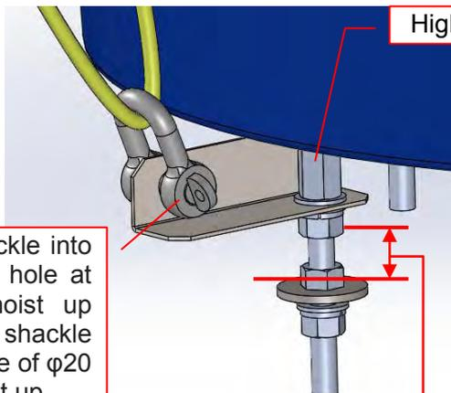
Hook shackle into lifting tool hole at  $\phi 20$  to hoist up
