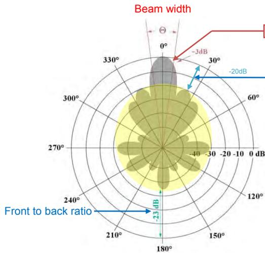
Figure 1.5: Antenna pattern in a polar-coordinate graph
