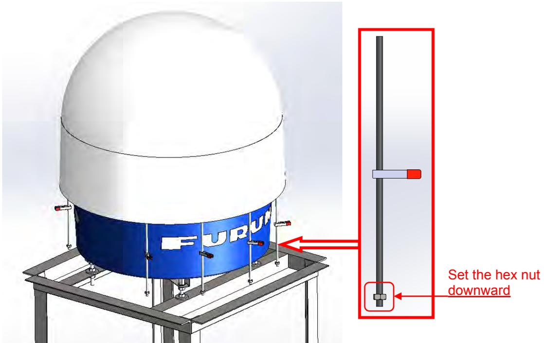
Figure 5.5: This image example uses 8 bolts.
