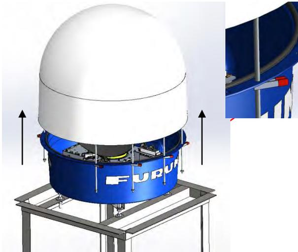
6. Remove spring clamp from bottom of radome and reattach it at top of the flange.
