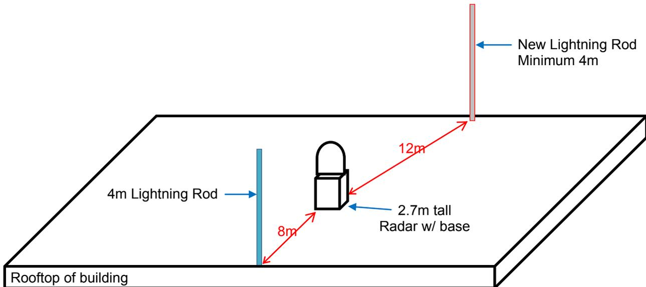
Figure A-4: Drawing at rooftop and candidate place to install the new lightning rod
