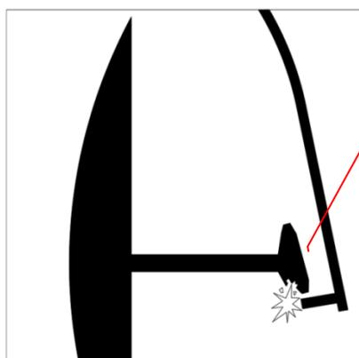
Caution: Move antenna to position feed arm vertically to ensure no contact when lifting radome top.
