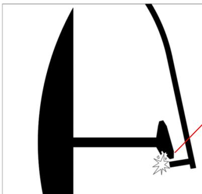
Avoid contact between the antenna feed arm and the radome internal flange when lifting radome top.
