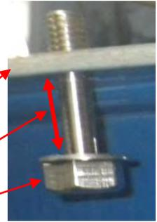
2. Lift up the radome slightly and rotate it counterclockwise around 30 degrees, the fixed hex nut will fit in to the recess part of top radome. The nut insert can be seen from the thru hole.
