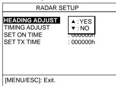
Radar setup menu (heading adjust)
