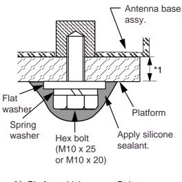
\*1: <u>Platform thickness</u> 5 mm or less: M10 x 20 5-10 mm: M10 x 25 over 10 mm: locally supplied bolts
