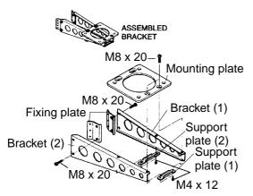
(A) Assembling the mounting bracket
