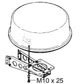
(B) Fastening antenna to mounting bracket
