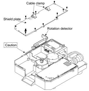
7. Pass the antenna cable with connector through the gasket and cable clamp, and then tighten the cable gland.
