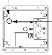
Make a hole of  $\phi$ 16. Seal hole with sealing compound after connecting cable.
