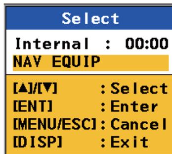
4. Select [Internal] or [NAV EQUIP] then press the **ENT** key. Select [Internal] to use local time, or [NAV EQUIP] to use UTC time. For [Internal], the [Local Time ADJ] screen appears; go to step 5. For [NAV EQUIP], go to step 6.
