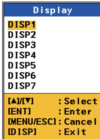
4. Select the display number (default display number for the graphic display is DISP5) where to show the speed graphic display then press the **ENT** key.
