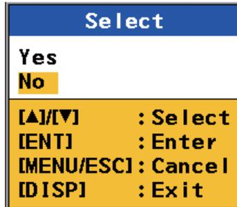
4. Select [Yes] then press the **ENT** key. All berthing lines in the sub display units are replaced with the berthing lines from the main display unit.
