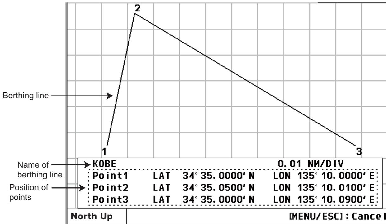
14. To save the line, press the **MENU/ESC** key to return to the [SET] dialog box (see the figure at the top of page 3-9). Press ▼ to show and select [Exit] then press the **ENT** key. (The berthing line is sent to all active sub display units when the **ENT** key is pressed.)
