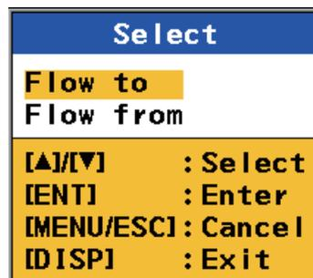
4. Select [Flow to] or [Flow from] then press the **ENT** key.
