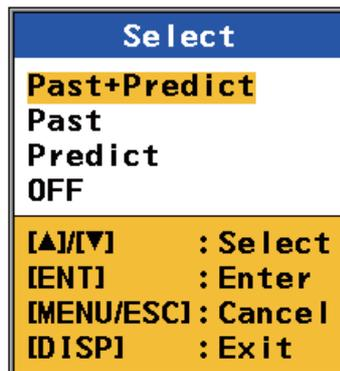
3. Select the type of track to display then press the **ENT** key. Select [OFF] to hide all tracks.
