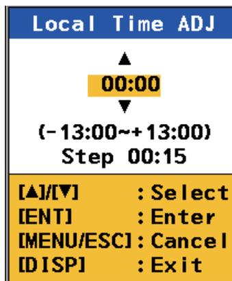
5. Use **▲**, **▼** to set the time difference between local time and UTC time then press the **ENT** key.
