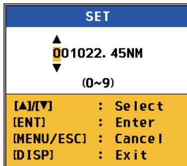
4. Use ▲ or ▼ to set a value then press the **ENT** key. (You can move the cursor to the right with the **ENT** key. Use the **MENU/ESC** key to move the cursor to the left.)
