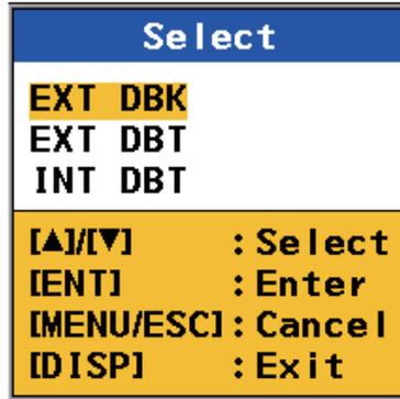
4. Select desired depth measurement reference then press the **ENT** key.
