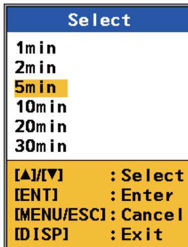
3. Select a time then press the **ENT** key. A new marker is plotted at equally time-spaced intervals of 1/5 of the plot time selected. For example, if you select the 10-minute interval, the predicted position is plotted at two-minute intervals.
