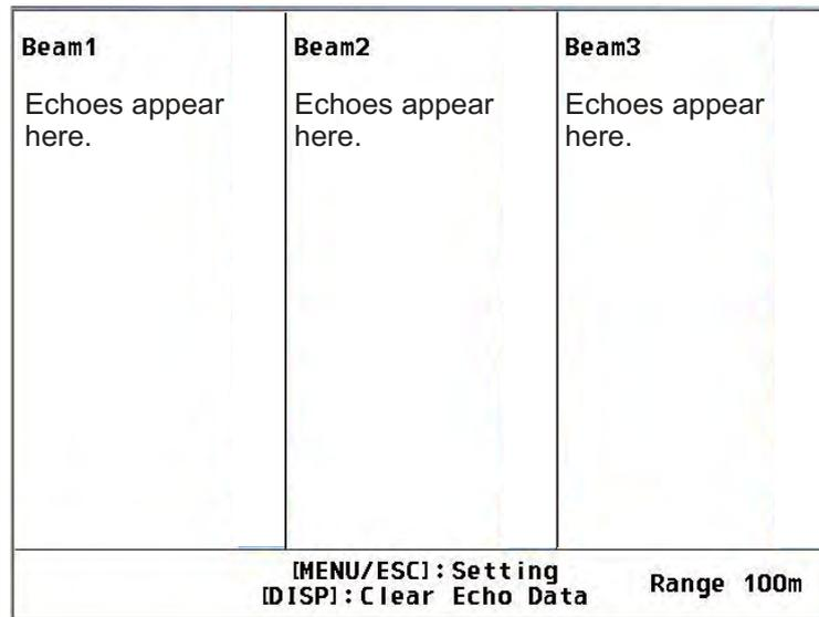
5. To change the range, press the **RNG** key. The available ranges are (in meters) 5, 10, 20, 40, 100, 200 and 300. The current range is shown at the bottom right corner on the echo monitor display.
