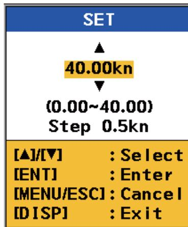
4. Press **▲** or **▼** to set the maximum allowable speed then press the **ENT** key. The setting range is 0.05 to 40 kn, in 0.5 kn increments.
