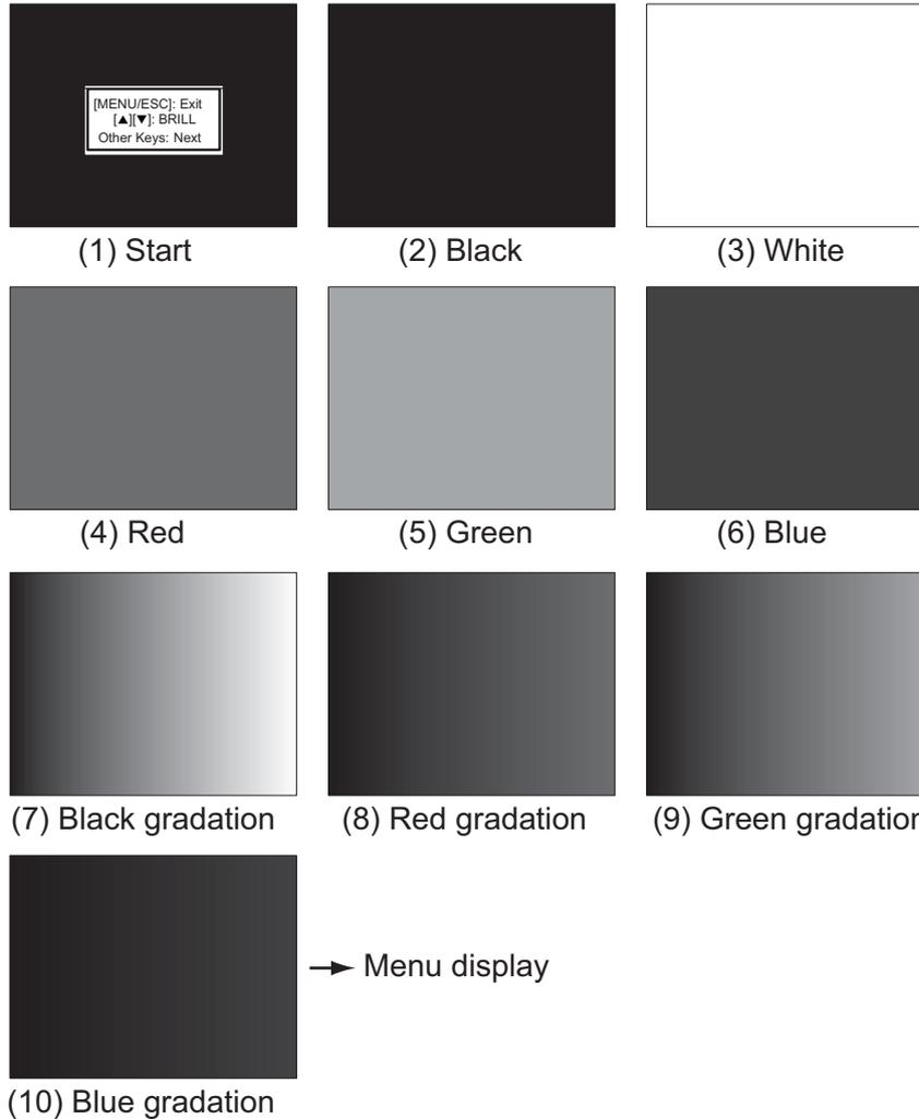
5. Control is returned to the menu after the blue gradation is shown. Press the **DISP** key to close the menu.
