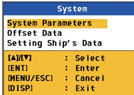
3. Select [System Parameters] then press the **ENT** key.
