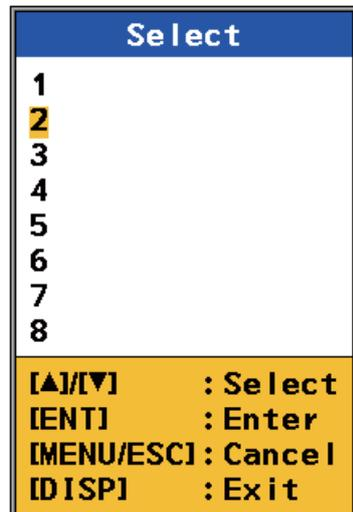
3. Select a dimmer level then press the **ENT** key. The higher the figure, the higher the dimmer level.
