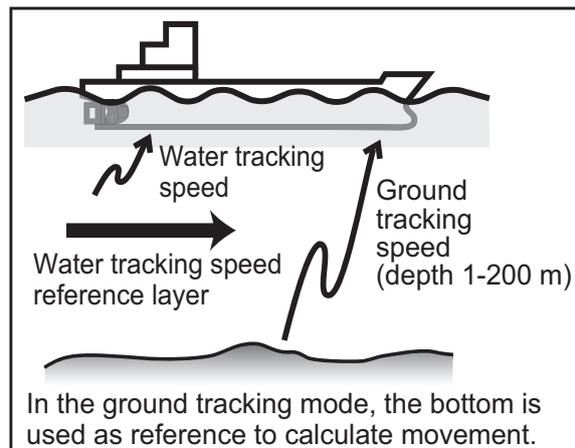
**Auto:** Automatically selects ground tracking mode or water tracking mode according to the depth. The water tracking mode is selected when the keel clearance is 200 m or more. (Actual working depth in the ground tracking mode depends on the bottom and water conditions, and the reflection properties for sonic pulses.)
