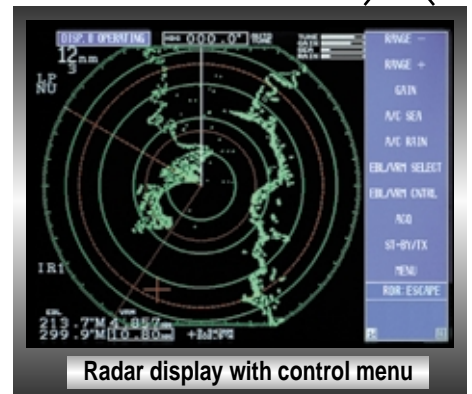
Radar control menu
