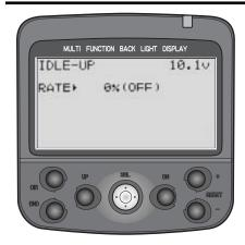
**DEFINITION:** Adjusts the throttle's idle/neutral point, usually used to create a raised idle, making it easier to start the engine. May adjust either toward higher idle (U) or toward braking (D).
