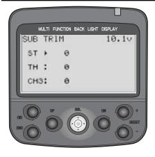
**DEFINITION:** Fine tuning adjustment for the center point of each servo. Similar to using electronic trims on the radio, but subtrim moves the entire servo's travel rather than just sliding the servo left/right within the total travel. The setting is stored within the programming and the onscreen displays continue to show neutral.
