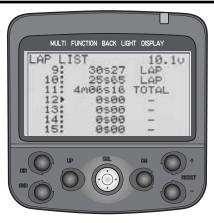
**DEFINITION:** Displays all stored lap times, up to 100, and also stores total race time, including run time after last but before reset/stop.
