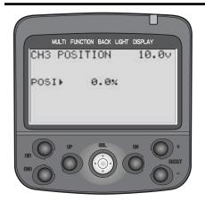
**DEFINITION:** Sets the default or neutral position for the channel 3 servo. Defaults to being adjustable with dial 3.
