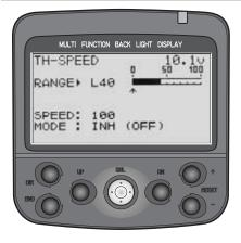
**DEFINITION:** Speed Limiter decreases the maximum speed of the servo. This may be adjusted individually for turning and returning the servo to neutral (steering), and for high and low throttle settings.
