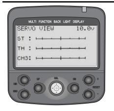
**DEFINITION:** Shows the exact outputs the transmitter is sending to the servos. Allows for easy testing/experimenting even when receiver and servos are not yet installed.
