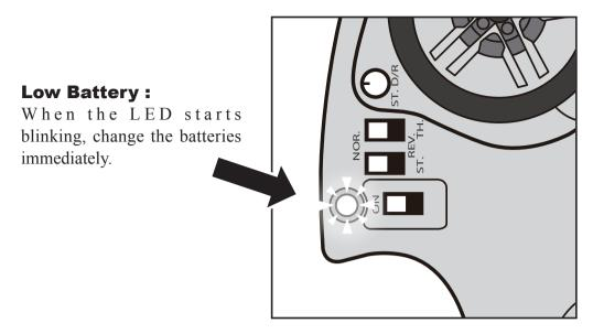
The low battery alarm is meant to be a safety feature only. Do NOT operate your radio below low battery. Always shut your radio off as soon as possible after the low battery warning tone to avoid loss of control.
