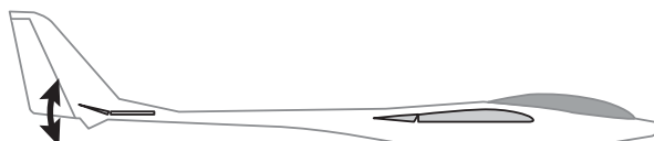
Only an elevator moves in case of a little operation.
