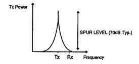
The normal setting is such that the gain is lower than the isolation by a 10dB margin. A larger margin accounts for environmental, aging and other changes in the system.
