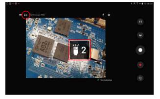
Brightness is 0 to 3 levels and is displayed on the screen. 0 is the LED is off.
