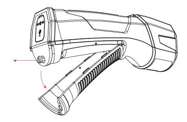
Remove the rechargeable battery and replace it with a new one.
