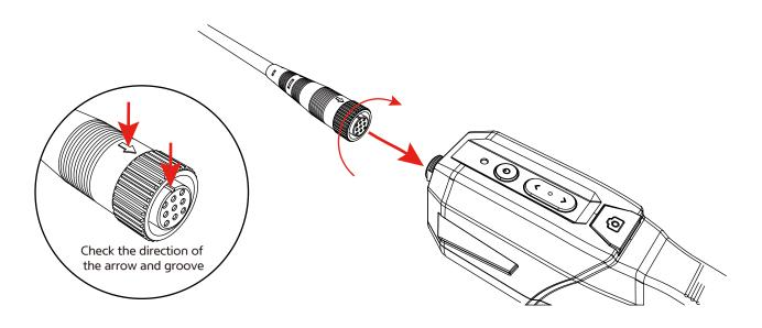
2 Insert the camera on the other side of the flexible tube and turn it to fix it.
