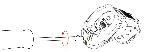
(2) Remove the screw and detach the battery cover on the handle part downward.
