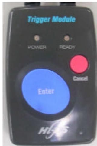
[Figure 3. Switches and LEDs of trigger module ]
