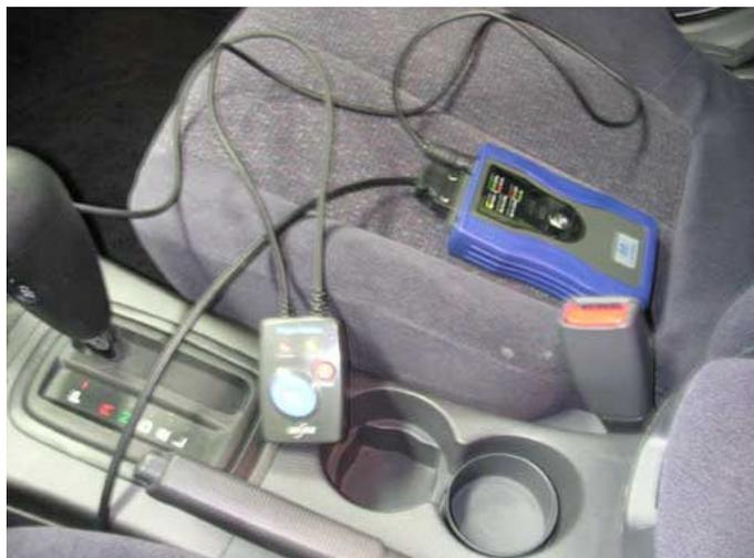
[Figure 1. Installation of trigger module]
