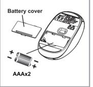
Remove the battery cover from the keyboard.
