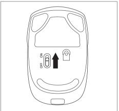
► Set the switch on the bottom of the mouse to "On".
