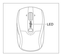
If the charge of the battery in the mouse becomes low, the LED on the mouse flashes red.
