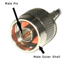
Test for DC short between male pin and outer shell of antenna connectors
