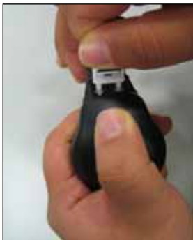
Figure 15: Inserting Retaining Pin
