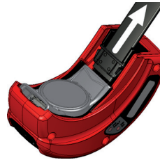
Figure 2 Pull on free end of strap
