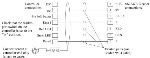
After wiring, re-attach the front cover and bezel.
