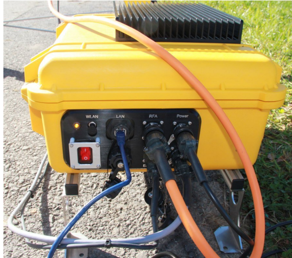
Figure 11: Instrument Controller and Power Unit in Pelican case. Connectors upper line from left to right: WLAN (not connected), Ethernet, RF Unit, Power. Lower line from left to right: Instrument Power Switch, USB, Motor Control, Motor Power.
