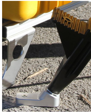
Figure 3: Tripod foot with special tip that allows screwing to the ground.
