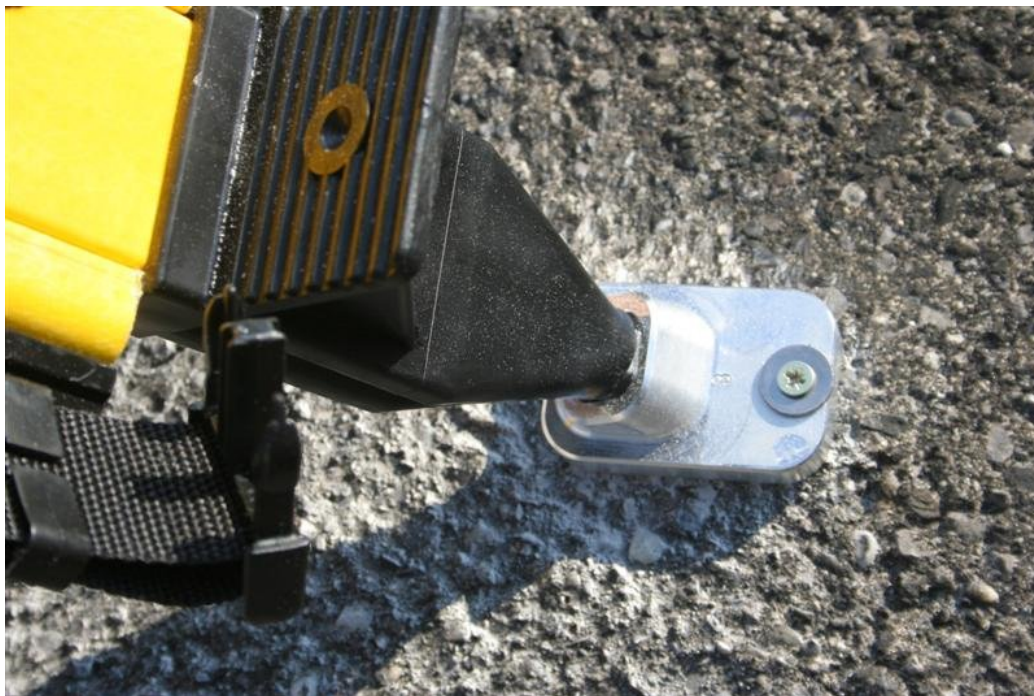
Figure 17: Tripod mounting adapter for screw anchor mounting.
