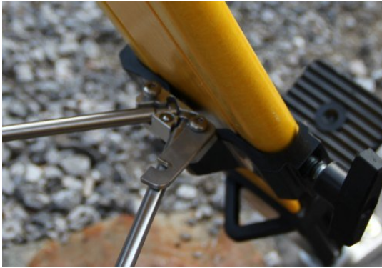
Figure 2: Fixture of rods to have tripod legs at fix distance.
