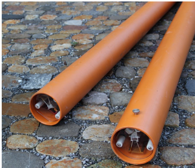
Figure 13: Antenna in the plastic tube containers. The antenna needs to be pushed out with the antenna side with the SMA connector in front.
