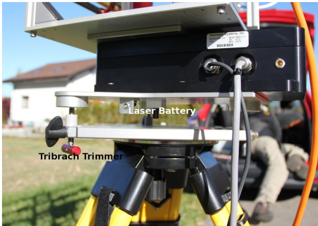
Figure 6: Side view of the Tripod - leveler - positioner - Antenna Tower setup. The leveler is adjust by rotating the red knobs. The black screw is to fix the knob setting. At the bottom of the motor, the connector for the laser battery is indicated.
