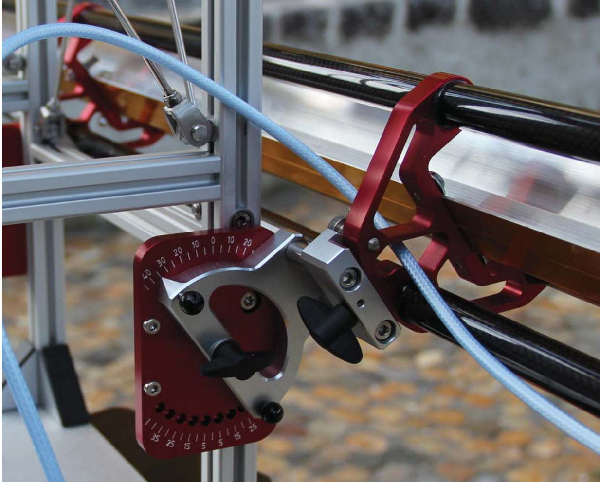
Figure 11: Closeup of the antenna bracket with elevation setting. Here an elevation angle of 35 degrees has been selected. Note that the angles in 10 degree steps are for the upper pin, and the angles offset by 5 degrees are on the lower circle.
