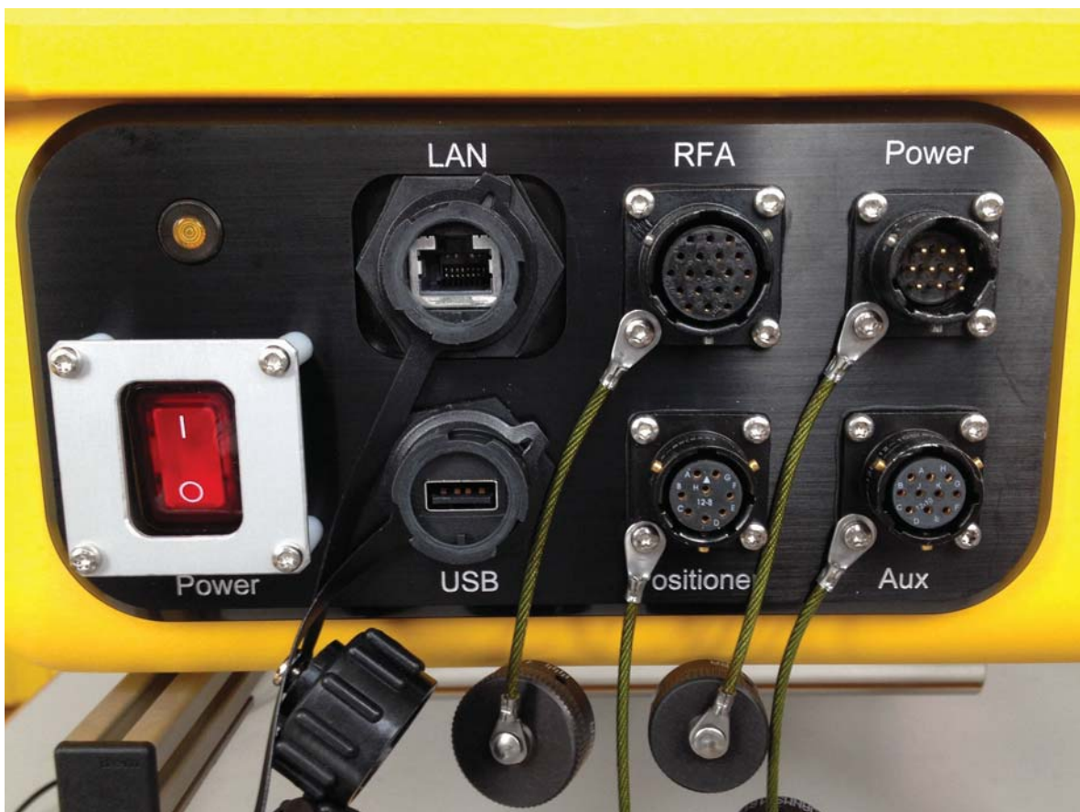
Figure 12: GPRI Connector Plate: Ethernet LAN, RFA, Power, USB, Scanner, Auxiliary Power for the radome fan connection
