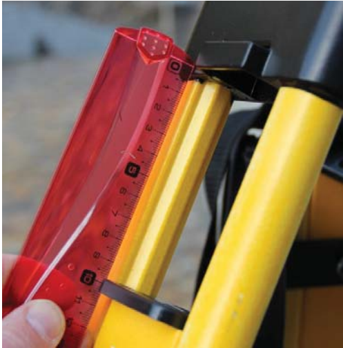
Figure 4: Tripod leg extent measurement. Only required for repeat measurements.
