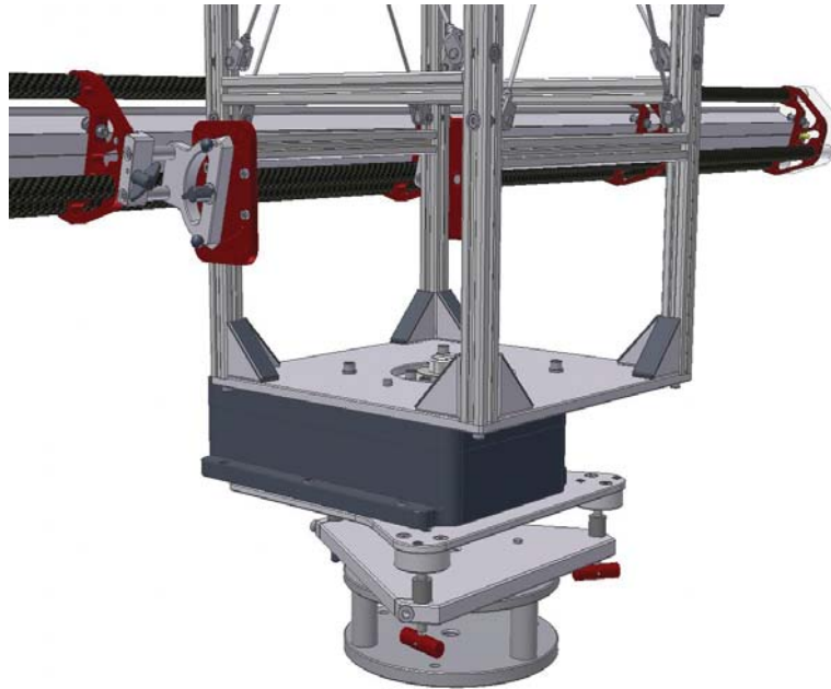
Figure 17: Tribrach with azimuthal scanner and tower. Adapter for pier mounting is shown attached to the tribrach. Red knobs adjust the tilt of the azimuthal scanner mounting plate.
