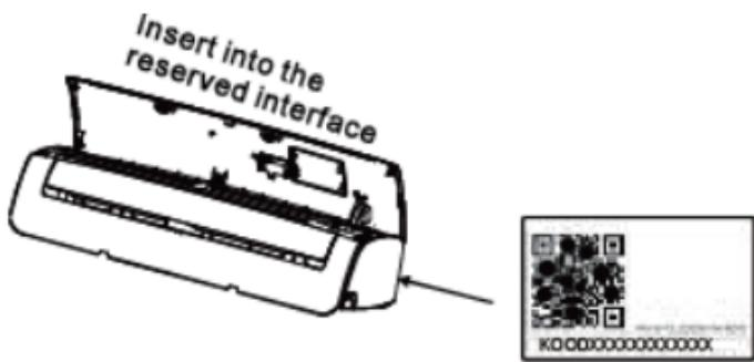
**WARNING:** This interface is only compatible with SMART KIT(Wireless module) provided by the manufacturer.
