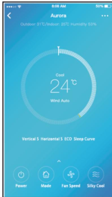
③ Thus, user can control air conditioners on/off status, operation mode, temperature, fan speed and so on.
