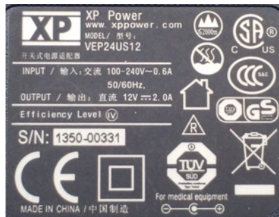
Figure 2-4. Vscan Extend AC/DC adapter label
