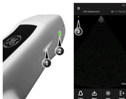
Figure 5-2. Dual probe: Orientation mark, phased array active
