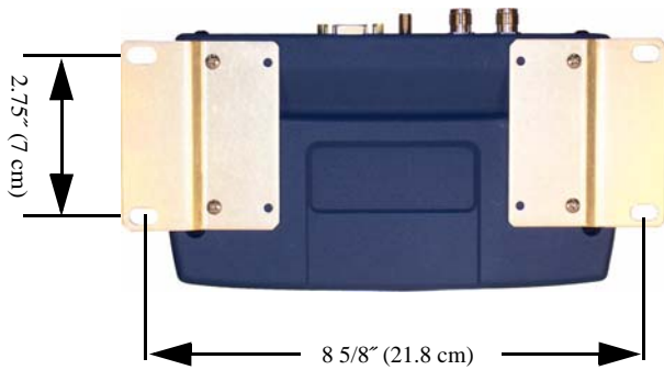
Figure 4. Transceiver Mounting Dimensions (Dimensions for BS and SU identical)
