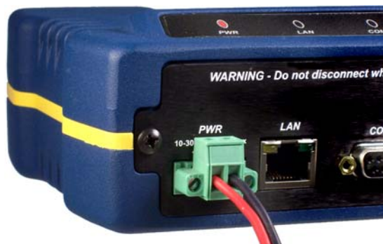
Figure 2-2. Power Connector (Polarity: Left +, Right −)
