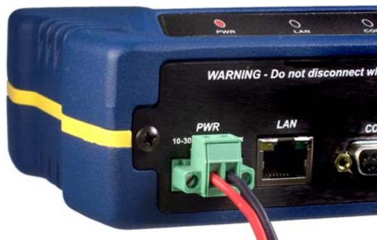
Figure 2-2. Power Connector (Polarity: Left +, Right –)
