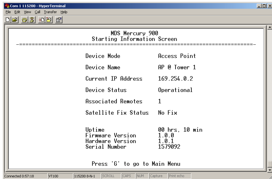
Figure 3-2. View of MS with a text-based program— (Console Terminal shown—Telnet has similar appearance)
