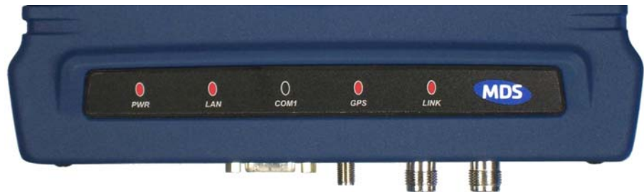
Figure 2-4. LED Indicator Panel
