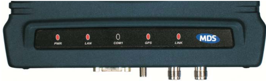
Figure 2-4. LED Indicator Panel
