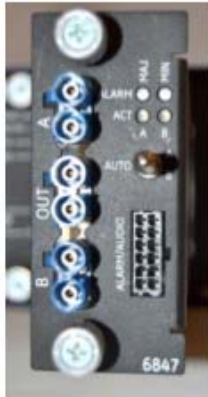
Figure 6-8 Alarm/Relay Module (Part No. 03-6847Axx; 03-6848Axx)
