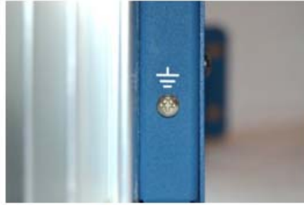
Figure 3-2. Rear Panel Grounding Screw
