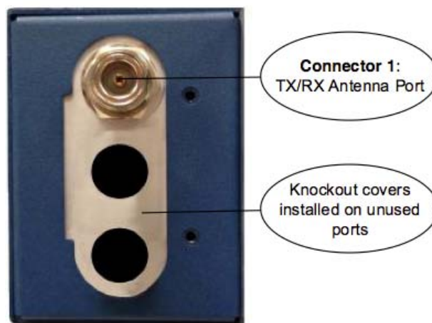
Figure 4-2. Internal Duplexer (or internal T/R switch), Single N connectors
