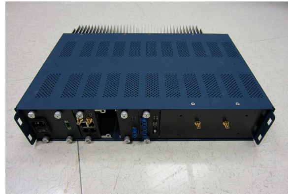
Figure 2: Typical Orbit Master Station Chassis. The SDM9 modules may be installed in any free peripheral slot of this chassis.
