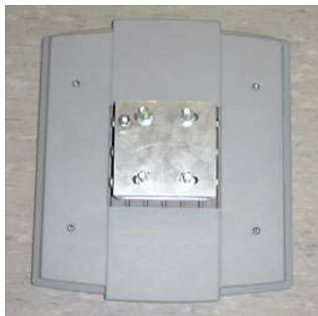
Figure 3-7. MDS FOUR.9 Series ODU Rear View
