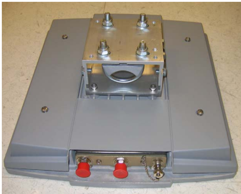
Figure 3-9. MDS FOUR.9 Series ODU with Mounted Tilt Bracket
