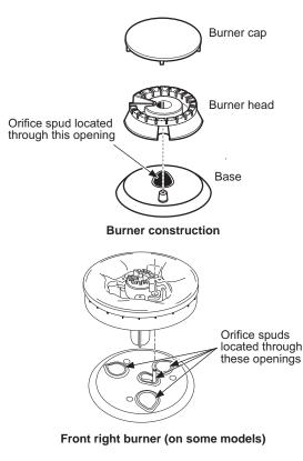
B. Using a 7 mm or 9/32" nut driver, remove the top burner orifices. These may be accessed through the burner opening in the base.
