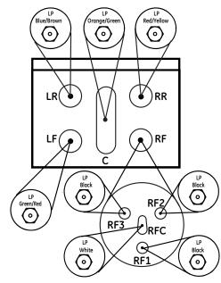
To prevent leakage, make sure the orifice spuds are securely screwed into the gas supply tubes.
