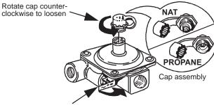
Lever shown closed (Oven Shut Off only) PUSH LEVER TOWARD REGULATOR TO OPEN
