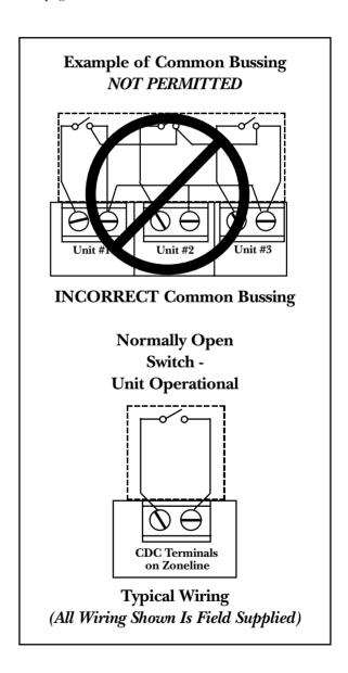
In some installations, control of the operation of the unit at a location remote to the unit itself may be desired. Unit mounting locations (high in the wall or over a transom) resulting in inaccessible unit mounted controls can be connected to a remote thermostat. Other installations may use remote thermostat control for design or performance enhancement. The unit is
