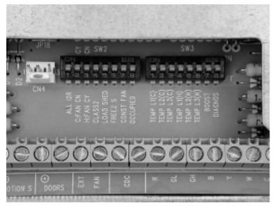
Cooling and Heating temperature limits are set independently. Temperature limiting switches in factory set down position except as noted.
