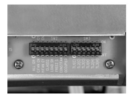
Cooling and Heating temperature limits are set independently. Temperature limiting switches in factory set down position except as noted.
