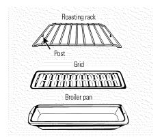
When you are convection roasting it is important that you use the broiler pan and grid and the special roasting rack for best convection roasting results. The pan is used to catch grease spills and the grid is used to prevent grease spatters.
