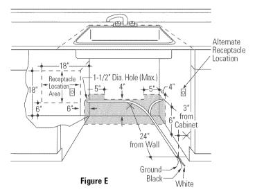
Cut hole 1-1/2" max. dia. within the shaded area to admit the
