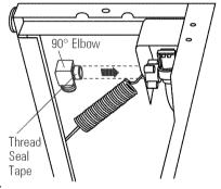
Do not bend the dishwasher frame when installing the 90° elbow fitting to the water
