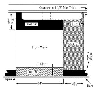
Sink opening for garbage disposer must be dimensioned as shown in Area "C." This will provide clearance for disposer and plumbing in cabinet "C" when using either single or
