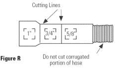
If the location requires a longer drain hose, add up to 42" of length to the factory installed hose. Use 5/8" or 7/8" inside diameter hose and a short section of copper water pipe of appropriate length and diameter to connect the two hose ends. Secure connection with appropriate clamps (not supplied).
