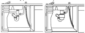
Waste tee installation Figure S Disposer Installation
