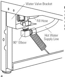
Important: When opening and closing the door, the door spring should not touch the fill hose. If it does, bend water valve bracket slightly to provide clearance between the spring and the fill hose.
