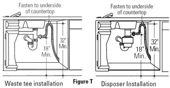
Note: BE SURE TO REMOVE DRAIN PLUG FROM DISPOSER BEFORE ATTACHING DRAIN LINE. DISHWASHER WILL NOT DRAIN IF PLUG IS LEFT IN PLACE.
